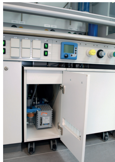
Stand-alone solution: Fine vacuum, Schlenk line
