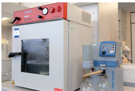
Drying cabinet with pumping unit
